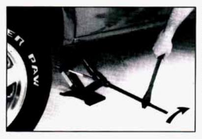
Raise the vehicle by rotating the ratchet clockwise. Make sure the UP marking faces you. Raise the vehicle far enough off the ground so there is enough room for the spare tire to fit.
